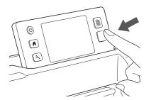
When cutting is finished, the message "Finished ► cutting." appears on the display. Touch the "OK" key to return to the draw/cut selection screen.
