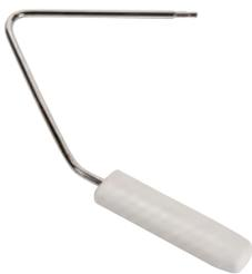
With the help of a knee lifter, the presser foot is lifted and the feed dog is lowered at the same time. This also increases the gap between stitch plate and presser foot, and leaves both hands free to guide your project.
