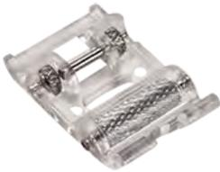
The Roller Foot is a specialist when sewing on difficult-to-feed materials. Thanks to its roller on the underside of the foot, it glides effortlessly over materials such as leather and vinyl, as well as fabrics with a strong surface structure.
