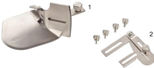
With the single fold binder attachment, fabric edges and necklines can be perfectly bordered with bias tape. The unfolded tape is inserted through the attached guide rail, folded over on the upper side while the under side remains open, and is then sewn on with a cover stitch. For the perfect look, the bias tape can also be self-made. Tapes of 40 mm width result in a finished width of approx. 10 mm. An attachment adapter is required to use the binder attachment.
