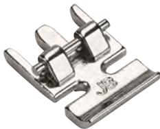
The Zipper Foot for Dual Feed features a recess on the rear side of the presser foot to activate the integrated dual feed. This ensures a consistent feed with multiple layers of fabric and difficult-to-feed materials.
