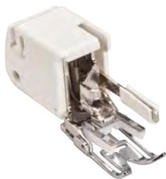
Fabrics that are difficult to work with are best sewn with the Walking Foot. It supports the fabric feed with a second feed dog on the top of the foot. The sewing project is moved in synchronization with the lower feed dog to ensure a smooth sewing process.
