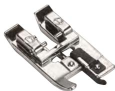
The Overlock Foot for Dual Feed features a recess on the rear side of the presser foot to activate the integrated dual feed. This allows an even feed with several layers of fabric. With elastic fabrics, the waving of the seam is reduced.
