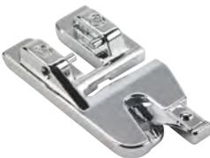
The Hemmer Foot for Dual Feed features a recess on the rear side of the presser foot to activate the integrated dual feed. This ensures a consistent feed with multiple layers of fabric and difficult-to-feed materials.
