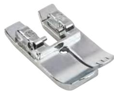
The Straight Stitch Foot for Dual Feed features a recess on the rear side of the presser foot to activate the integrated dual feed. This ensures a consistent feed with multiple layers of fabric and difficult-to-feed materials.
