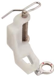
The Hopper Embroidery Foot is the perfect choice when embroidering on pile and bulky fabrics, such as terrycloth. Due to the spring mechanism, the material to be embroidered is optimally pressed down, and at the same time, the movability of the foot compensates for uneven areas, such as with puffy fonts or multi-layer quilts, which results in a beautiful stitch formation.
