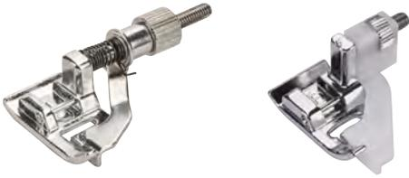
This foot is best suited to sew blind hems or to topstitch edges. The stitches only pierce the hem so that the stitch holes are hardly visible on the right side of the fabric.
