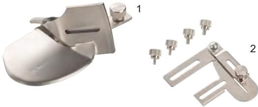
Due to the top bottom double fold binder attachment, fabric edges and necklines can be perfectly bordered with bias tape. The unfolded tape is inserted through the attached guide rail, folded over twice on the upper and lower sides of the bias tape and sewn on with a cover or chain stitch. For the perfect look, the bias tape can also be self-made. Tapes of 36 mm width result in a finished width of approx. 10 mm. An attachment adapter is required to use the binder attachment.
