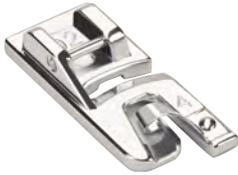
In order to create professional hems, this special presser foot is perfect. It wraps the fabric twice. This creates a narrow circular hem which is then neatly fixed with the straight stitch by the needle.
