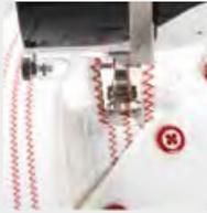
Mounting bracket for attaching the magnifying lens or PunchWork tool.
